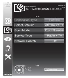
9 Select the line »Scan Mode« with »V« or »∧«. Select the scan mode with »≪« or »>« (for unencrypted channels, for encrypted)
